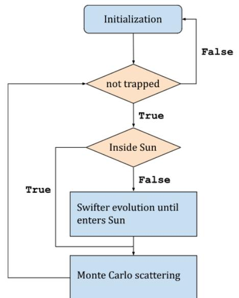
FIG. 5: Flowchart of `starcodes`
